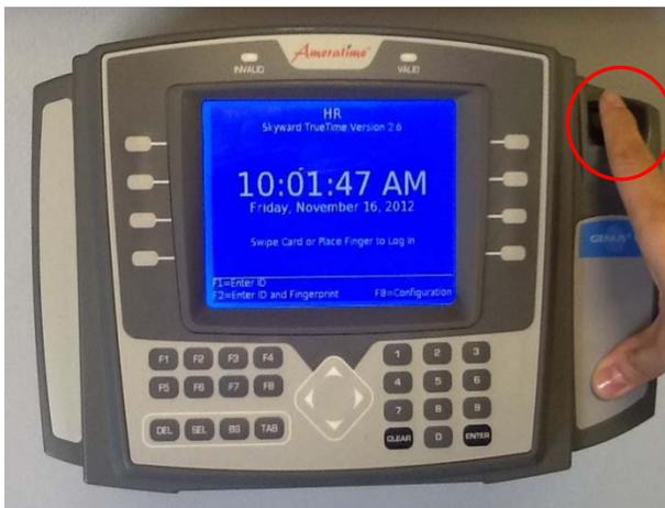
The fingerprint reader is on the upper right side of the biometric clock.
